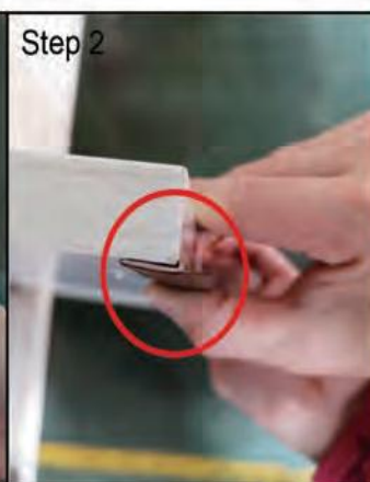
Step 2 卡角紧贴柜门边缘扣住 Clamp the corner close to the edge of the cabinet door
